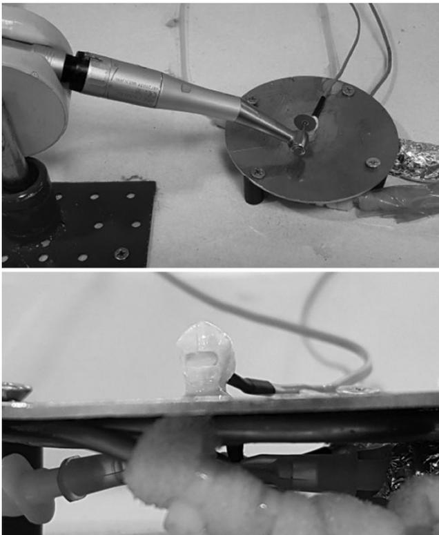
**FIGURE 1** Photo of the pulpal blood microcirculation model set-up (above). The inflow water heat stabilizer system (below)
